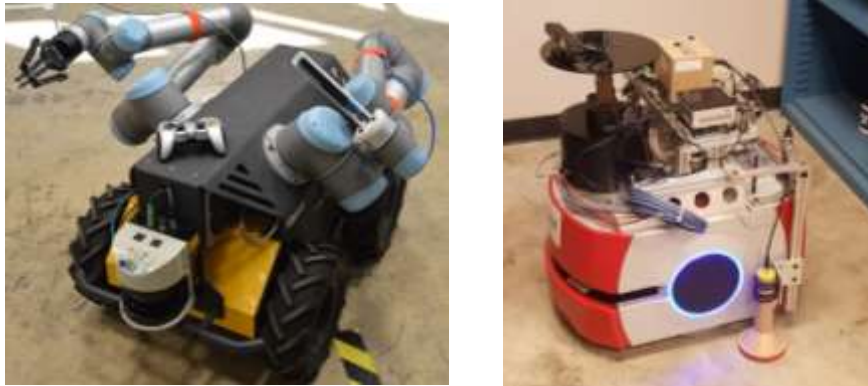
Fig. 1. Two robotic systems developed by UT Austin for LANL: (left) the “VaultBot” dual-arm mobile manipulator and (right) the Pioneer LX Platform.
